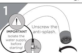
Remove the anti-splash from housing. Clean and replace as necessary.
